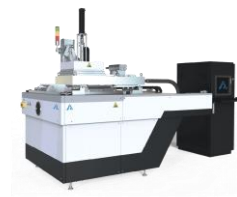
DIAMANTA vacuum system with PECVD technology
